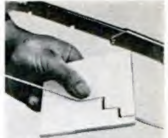
Rod Saw. Thin, round blade cuts in any direction. Ideal for contour cutting. Reversible for extended life. Ten-inch length fits standard hacksaws.
